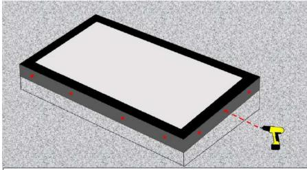
${\bf 9} \ \, \text{Pre drill fixing holes through aluminium and timber upstand/kerb at 100mm from each corner and then at regular intervals.}$
